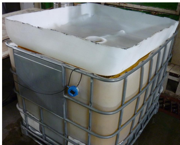
Semi-commercial hot water treatment trial unit at NWC. Papaya dipped in 48° C water for 20 minutes has shown a reduction in post-harvest disease severity compared to untreated fruit.
